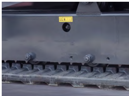
Lower track roller Forged rollers offer upto 75% greater strength compared to cast items, improving their wear resistant properties.
