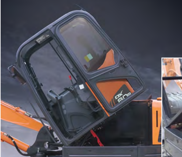
Tilting cabin for easy maintenance
