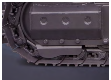
Fabricated Track Guide The track guides which protects the vital track components are fabricated components and can be easily replaced.
